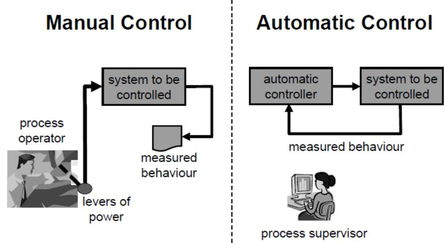
*Automatic control* describes the situation in which a machine is controlled by another machine.
