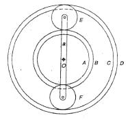
2. a) In an epicyclic gear of the sun and planet type as shown in figure. , the PCD of the internally toothed ring is to be 224 mm and the module 4 mm. When the ring D is stationary, the spider A, which carries three planet wheel C of equal size, is to make one revolution in the same sense as the sun wheel B for every five revolutions of the driving spindle carrying the sun wheel B. Determine the suitable number of teeth for all the wheels.
