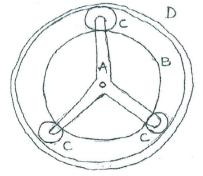
b) A punching press is required to punch 40 mm dia. Holes in a plate of 15 mm thickness at the rate of 30 holes per min. It requires 6 Nm of energy per mm<sup>2</sup> of sheared area. If punching takes 1/10 sec. and the rpm of the flywheel varies from 160 to 140. Determine the mass of the flywheel having radius of gyration of 1 meter.
